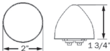
MC25 SERIES HOLE CUT-OUT: 2.313"
